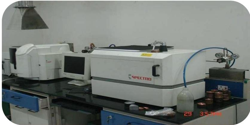
Atomic Absorption Spectrometer & Spark Emission Spectrometer
